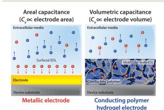
Fig. 14 Capacitive charge injection by metallic electrode materials relies on the formation of surficial EDL whose capacitance is proportional to the electrode area (areal capacitance). In contrast, capacitive charge injection by a conducting polymer hydrogel electrode relies on the formation of molecular-level EDL throughout the conducting polymer hydrogel whose capacitance is proportional to the electrode volume (volumetric capacitance).
