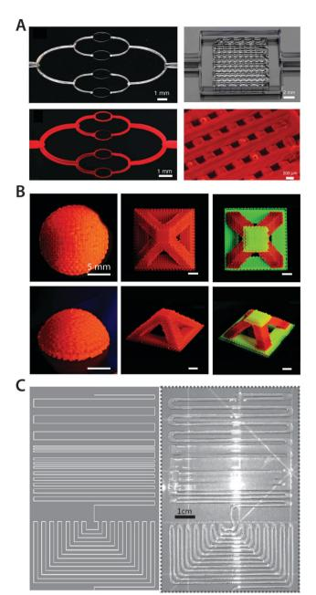
Fig. 21 Direct ink writing 3D printing of hydrogels. (A) 3D printed hydrogels with micro-scale vascular networks. Adopted with permission from ref. 208. Copyright 2014 Wiley-VCH. (B) Multi-material high resolution 3D printing of hydrogels into various geometries. Reproduced with permission from ref. 211. Copyright 2018 Wiley-VCH. (C) 3D printed ionically conductive hydrogel circuits on silicone elastomer substrate. Adopted with permission from ref. 209. Copyright 2017 Wiley-VCH.
