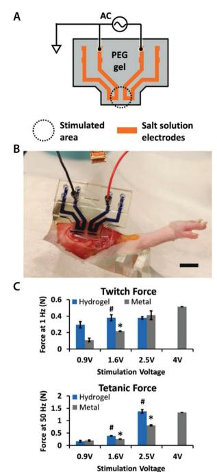
Fig. 9 Hydrogel ionic circuits for in vivo electrical stimulation of muscles. (A) Ionic salt solution encapsulated within the PEG hydrogel serves as an electrode. (B) The hydrogel ionic stimulating electrode is placed on the rat muscle with external electronic connections. (C) The hydrogel ionic stimulation electrode exhibits better or comparable muscular activation under stimulation inputs compared to standard gold electrodes. Reproduced with permission from ref. 98. Copyright 2018 Wiley-VCH.
