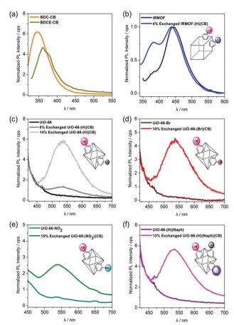
Fig. 2 Photoluminescence spectra of carborane-functionalized ligands and UiO-66s
