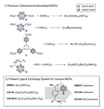
Scheme 1 Method of installing carborane into metal-organic frameworks.
