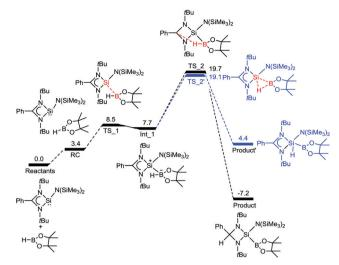
Fig. 2 The reaction free energy profile diagram for the B-H bond activation by 1. The values (in kcal mol<sup>-1</sup>) have been calculated at the PBE/TZVP level of theory.
