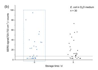
Fig. 5 (a) SERS signal at around 733 cm $^{-1}$  of *E. coli* with and without 25% D<sub>2</sub>O addition plotted against Raman shift (bars: 1 s); (b) SERS intensity of *E. coli* with 25% addition of D<sub>2</sub>O after 0 and 5 d storage. Note that the data at day 0 in the blue box of panel (b) corresponds to the deuterium data in the blue box of panel (a).
