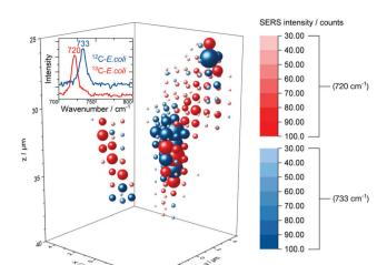
Fig. 7 3D SERS image of  $^{12}\text{C}/^{13}\text{C}$ -labelled *E. coli* cells embedded into an agarose matrix. Not shifted and red-shifted SERS signal are drawn at each grid position in blue and red spheres respectively, the size and saturation represent the intensity. The corresponding rotating iso-surface plot is available in the ESI.†
