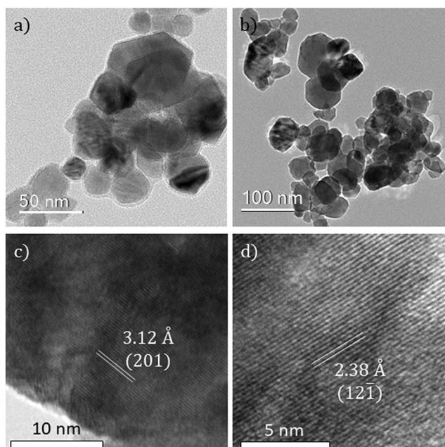
Fig. 4 TEM images of (a) undoped VO<sub>2</sub> and (b) Nb-doped VO<sub>2</sub>. Lattice fringes of (c) undoped VO<sub>2</sub> and (d) Nb-doped VO<sub>2</sub>.
