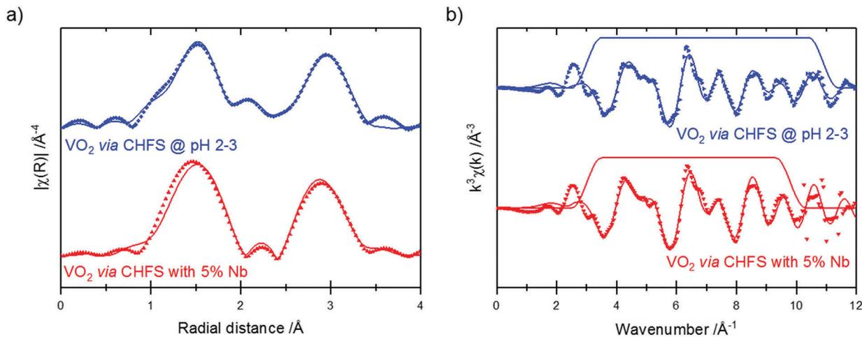
Fig. 7 V K-edge Fourier transforms (a) and EXAFS (b) of the CHFS VO<sub>2</sub> samples. Data are plotted as symbols, and fits as solid lines. The trapezoid lines in (b) indicate the Fourier transform window used.
