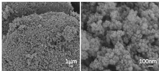
Fig. 3 SEM images of the un-doped VO<sub>2</sub>(M) powder.
