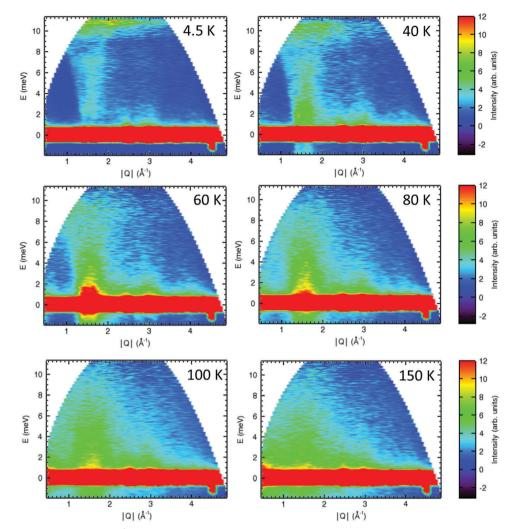
Fig. 8 Inelastic spectra collected at  $\lambda = 2.5$  Å for Ca<sub>2</sub>Mn<sub>3</sub>O<sub>8</sub> at variable temperatures.
