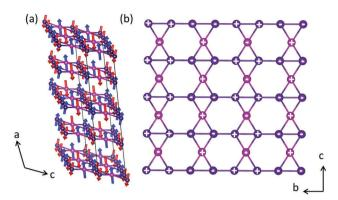
Fig. 6 (a) Magnetic structure of Ca<sub>2</sub>Mn<sub>3</sub>O<sub>8</sub> refined at 4 K showing the spin orientation between the MnO<sub>6</sub> layers in the a-direction (red is spin-up, blue is spin-down) and (b) the \\ \ \ \ \ \ \ \ \ spin arrangement on the Mn2 crystallographic site (purple) in the bc plane.
