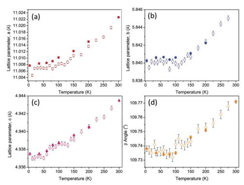
Fig. 4 Lattice parameters (a) a, (b) b, (c) c, and (d)  $\beta$  angle as a function of temperature showing a invariant effect in the lattice b-direction and  $\beta$  angle which persists up to a temperature of approximately 130 K. Open and closed symbols are XRD and neutron diffraction data respectively. Note: error bars indicate 1 standard deviation and in some data are smaller than the symbol size.
