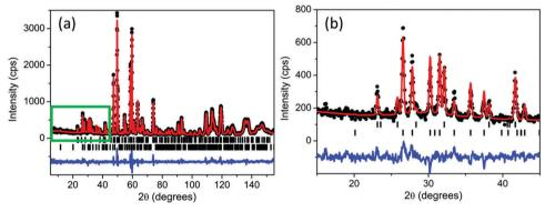
Fig. 5 (a) Rietveld refinement of neutron diffraction data collected for  $Ca_2Mn_3O_8$  at 4 K. Where the black circles are the observed data, the red line is the calculated model and the blue line is the difference curve. The bottom tick marks are the C2/m phase and the top tick marks represent the magnetic Bragg reflections. (b) Shows a zoomed in region at high d-spacing (as shown in the box in figure (a)) showing the magnetic Bragg peaks more clearly.
