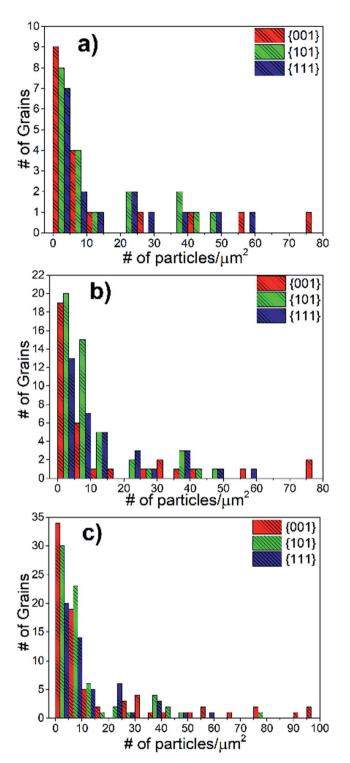
Fig. 8 The total distribution of precipitate number density on differently oriented grains at the surface of LSC64 pellets annealed at 800 °C for 2 h and 5 h. The grain orientations were processed with (a)  $10^{\circ}$ , (b)  $15^{\circ}$  and (c)  $17.5^{\circ}$  tolerance angles from the major orientations.
