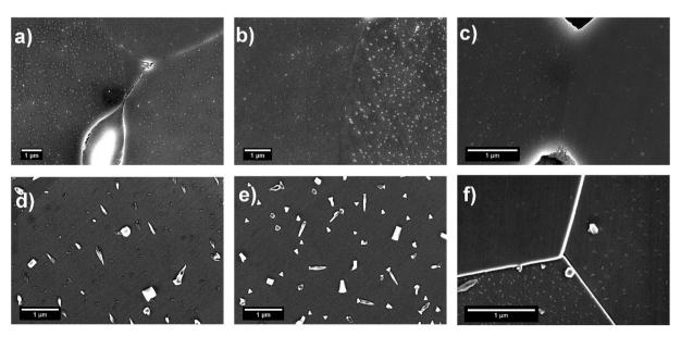
Fig. 3 SEM micrographs (secondary electron image mode) showing the grain dependence of secondary phase precipitate formation at the surface of LSC64 pellets annealed at 800 °C in stagnant air for 2 h (a-c) and for 5 h (d-f).
