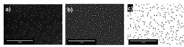
Fig. 7 (a) SEM secondary electron image of an area within a grain having some precipitates. (b) The same SEM image as in (a), with improved contrast upon applying the FFT filter. (c) The same SEM image as in (b), after performing background subtraction. The number density and area coverage of precipitates were calculated on the images after background subtraction.
