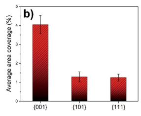
Fig. 10 (a) Average of precipitate number density and (b) average of precipitate area coverage on the three selected main orientations, {001}, {101} and {111}, at the surface of LSC64 pellets annealed at 800 °C for 2 h and 5 h.
