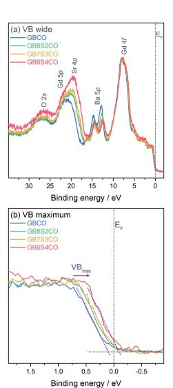
Fig. 6 X-ray photoelectron spectra of GBCO, GB8S2CO, GB7S3CO, and GB6S4CO, including (a) wide valence region, and (b) an expanded view around the valence band maximum VB<sub>max</sub>. Linear fits to the background and  $VB_{max}$  are shown as dotted lines in (b). The dotted line at 0 eV indicates the position of the Fermi energy  $E_{\rm F}$ .
