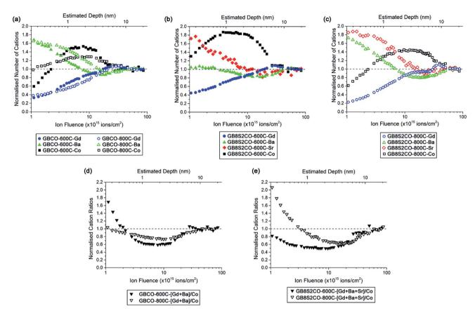
Fig. 7 Cation depth profiles obtained from low energy ion scattering (LEIS) spectroscopy (a) individual cations in GBCO, (b) individual cations in GB8S2CO annealed at 600 °C and (c) individual cations in GB8S2CO annealed at 800 °C, whilst (d, e) [Gd + Ba + Sr]/Co ratio in GBCO and GB8S2CO, respectively.
