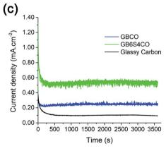
Fig. 9 (a) Linear sweep voltammetry at the 6<sup>th</sup> cycle and the corresponding (b) Tafel plot (at 1 mV s $^{-1}$  scan rate) in 0.1 M KOH electrolyte. (c) Chronoamperometry measurements of different GBSCO compounds at 1.65 V ( $\eta=420$  mV). Electrochemical measurements were iR compensated using current interrupt method. Higher performance was achieved with higher Sr dopant level.
