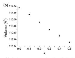
Fig. 4 (a) Lattice parameters of  $GdBa_{1-x}Sr_xCo_2O_{6-\delta}$  showing a decrease in a and b (for x = 0 and 0.1, 1/2b is used for comparison) parameters with increasing Sr dopant whilst c increases to x = 0.3 and decreases with x > 0.3. Dashed lines are plotted as a guide to the eye. (b) Volume decreases as x increases consistent with smaller ionic radius of Sr<sup>2+</sup> than Ba<sup>2+</sup>. Error bars are smaller than the symbols. Note transition to tetragonal at x = 0.4.
