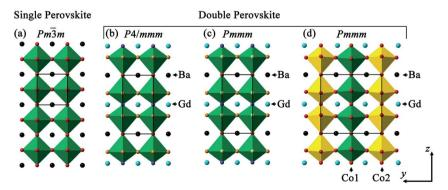
Fig. 1 Crystal structure representation of (a) single ABO<sub>3</sub> perovskite where A is represented in black and BO<sub>6</sub> polyhedra in green; and (b–d) double perovskite GdBaCo<sub>2</sub>O<sub>6</sub> where Gd<sup>3+</sup> (blue) and Ba<sup>2+</sup> cations (black) are ordered in z direction with (b) tetragonal P4/mmm, (c) orthorhombic Pmmm and (d) Pmmm with additional ordered cations along b depicted by Co1O<sub>6</sub> (green) and Co2O<sub>6</sub> (yellow) octahedra ordering.
