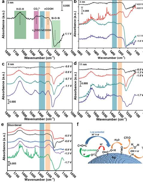
Fig. 4 (a) ATR-SEIRAS spectra of 3 nm Ag in  $CO_2$  saturated 0.1 M KCl electrolyte at -1.1 V. ATR-SEIRAS spectra of (b) 3 nm, (c) 5 nm, (d) 11 nm and (e) disordered Ag in  $CO_2$  saturated 0.1 M KCl electrolyte at different potentials. (f) Reaction mechanism for the  $CO_2$ RR and HER on the Ag surface.
