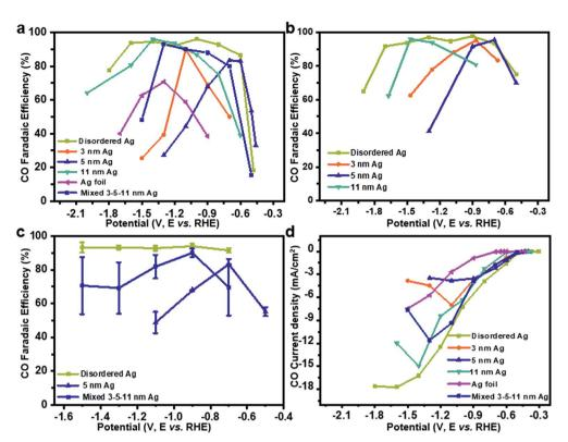
Fig. 2 CO faradaic efficiency depending on applied potential in  $CO_2$  saturated (a) 0.1 M KHCO<sub>3</sub> and (b) 0.1 M KCl, (c) CO faradaic efficiency on a simple mixture of 3–5–11 nm, disordered and 5 nm Ag in 0.1 M KHCO<sub>3</sub> with error bars. (d) CO partial current density depending on applied potential
