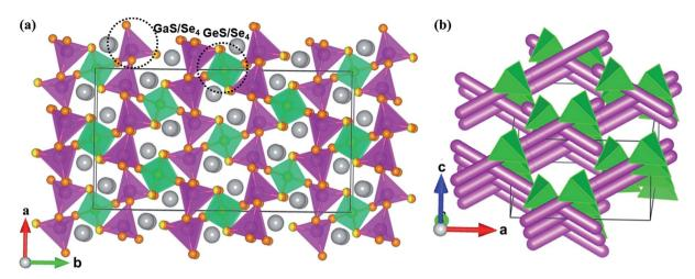
Fig. 1 (a) The 3-D structure of 1 viewed down the c direction. Grey atoms: Na, pink tetrahedra:  $[Ga(S/Se)Se_3]^{5-}$ , green tetrahedra:  $[Ge(S/Se)_2Se_2]^{4-}$ ; yellow/orange atoms: S/Se atoms. (b) The infinite  $_{\infty}^{1}[Ga(S/Se)Se_2]^{3-}$  chains represented by pink columns and isolated  $[Ge(S/Se)_2Se_2]^{4-}$  connections (green tetrahedra) in the unit cell of 1. The Na<sup>+</sup> cations are left out for clarity.
