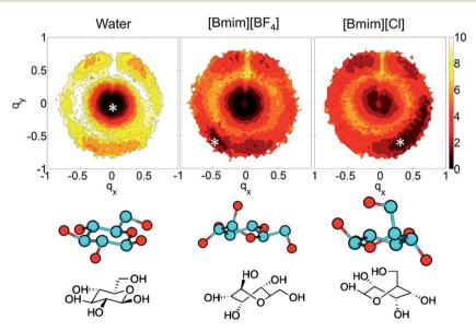
Fig. 15 The free energy distribution of the glucose ring conformation in the three solvents.  $q_{x,y}$  is the wrinkle coordinate, and the color depth represents the probability density. The bottom part below the snowflake symbol is the glucose configuration.<sup>87</sup> Reproduced from ref. 87 with permission from the American Chemical Society.
