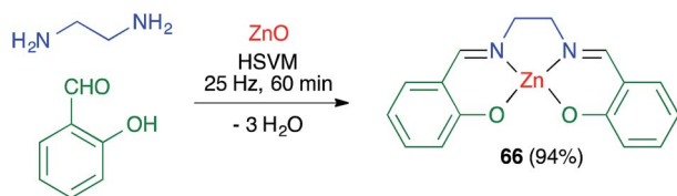
Scheme 46 Mechanochemical synthesis of a zinc-salen complex.
