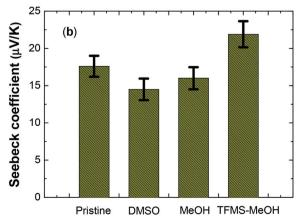
Fig. 2 Electrical conductivity (a) and Seebeck coefficient (b) of PEDOT:PSS thin films with different solvent treatment.
