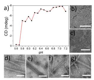
Fig. 2 (a) pH-dependent CD signal intensity at 583 nm of SBA/R3GN after incubation for 24 h at 4  $^{\circ}$ C ([SBA]: 0.1 mM, [R3GN]: 0.2 mM). (b–g) TEM images of SBA/R3GN stained by uranyl acetate at different pH from 5.6 to 6.1 (from b to g) with 0.1 interval. Scale bar: 200 nm.
