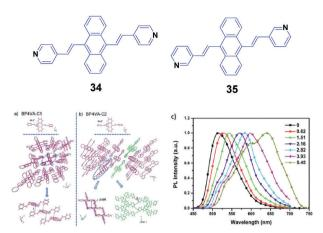
Fig. 11 (Top) The molecular structures of compounds 34 and 35. (Bottom) The aggregation state of 34 in the two single crystals: (a) C1 and (b) C2. (c) Normalized solid-state PL spectra of the 34 powder after the application of pressure (GPa). Reproduced with permission from ref. 52. Copyright 2013 The Royal Society of Chemistry.
