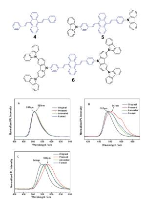
Fig. 4 (Top) The molecular structures of compounds 4, 5 and 6. (Bottom) The normalized PL spectra of 4 (A), 5 (B) and 6 (C) samples obtained under different conditions. Original: original sample; ground: ground sample; annealed: after annealing the ground sample at 200  $^{\circ}\text{C}$  for 5 min; and fumed: after fuming the ground sample in CH<sub>2</sub>Cl<sub>2</sub> vapor for 5 min. Reproduced with permission from ref. 32. Copyright 2012 American Chemical Society.
