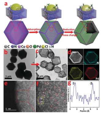
Fig. 1 (a) Schematic illustration of the preparation of Pd<sub>1</sub>/H-ZIF, (b) TEM image of ZIF-67, (c) TEM image of Pd<sub>1</sub>/H-ZIF, (d) corresponding EDS mapping images of N, C and Pd, (e and f) magnified HAADF-STEM images of Pd<sub>1</sub>/H-ZIF, showing that only Pd atoms are present in Pd<sub>1</sub>/H-ZIF, and (g) the corresponding intensity profiles obtained on the yellow area in (f).
