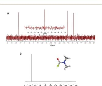
Fig. 8 (a)  $^{19}$ F NMR spectrum (in DMF, 470 MHz) of the supernatant liquid obtained from a FG/DMF suspension heated at 120  $^{\circ}$ C for 5 hours and stirred at room temperature overnight (in the inset, a close-up of the peak at -26 ppm is shown). (b)  $^{19}$ F NMR spectrum (in DMF, 470 MHz) of the separately prepared compound F-DMF (structure shown in inset). (b)  $^{19}$ F NMR spectrum (in DMF, 470 MHz) of the separately prepared compound F-DMF (structure shown in inset).
