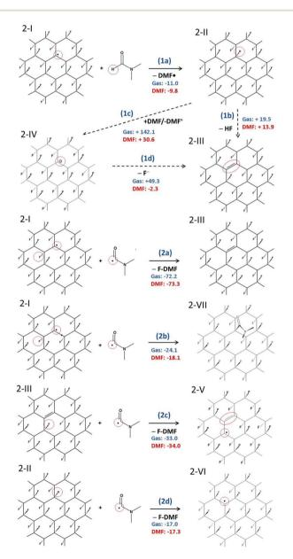
Fig. 3 Radical mechanism of defluorination of FG in DMF. (1a-c) Initial phases of defluorination. (2a-d) Re-creation of FG radical center. The reaction energies are given in kcal mol<sup>-1</sup>.
