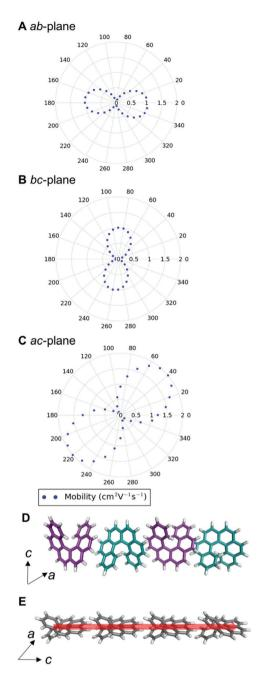
Fig. 7 Angular-dependent hole-mobility for structure 4 in the (a) ab-, (b) bc- and (c) ac-planes; (d) the adjacent heterochiral chain (substructure type IX) with hole-mobility of 0.01 cm<sup>2</sup> V<sup>-1</sup> s<sup>-1</sup> (e) the herringbone translational homochiral chain (substructure type X) with hole-mobility of 2.0 cm<sup>2</sup> V<sup>-1</sup> s<sup>-1</sup>. The red arrow shows the highest hole-mobility direction for structure 4.
