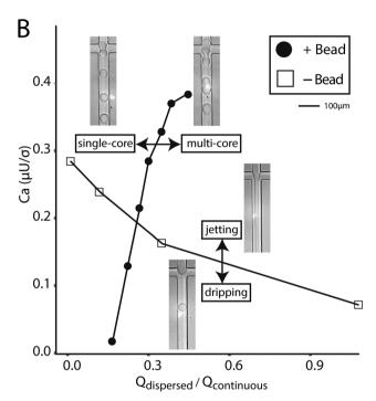
Fig. 4 Bead-dependent drop formation in the jetting regime without an aqueous co-flow. A) Microscope images of single-bead and multibead containing drops. B) Phase diagram of the transition from single-to multi-bead drops as a function of capillary number and flow rate ratio. Images of devices depict operation in particular regions.
