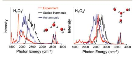
Fig. 1 Calculated spectra obtained using the approach described in the text. Comparisons are made to the argon-tagged spectra reported in ref. 3.
