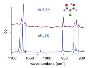
Fig. 4 Infrared spectra of MACl in pH<sub>2</sub> (bottom) at 5 K and in Ar (top) at 8.6 K in the spectral range of the doublets described in the paper (Fig. 7). The black dotted lines and brackets highlight the doublets discussed as associated with the tunneling splitting of vibrational levels.
