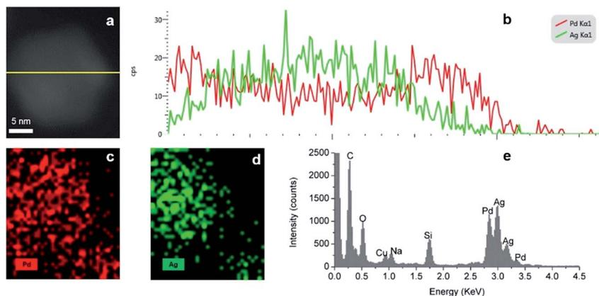
Fig. 14 (a and b) EDS line scan, (c and d) EDS elemental mapping and (e) EDS spectra of Ag–Pd alloy NPs synthesised by simultaneous reduction of  $\text{Ag}(\text{NO}_3)_3$  and  $\text{Pd}(\text{NO}_3)_2$  with HQ.
