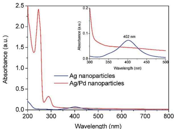
Fig. 5 UV-vis spectra of Ag nanoparticles after Reactor 2 and Ag–Pd bimetallic nanoparticles after Reactor 3 when  $\text{Pd}(\text{NO}_3)_2$  is used as precursor. All the solutions were diluted 12 times.
