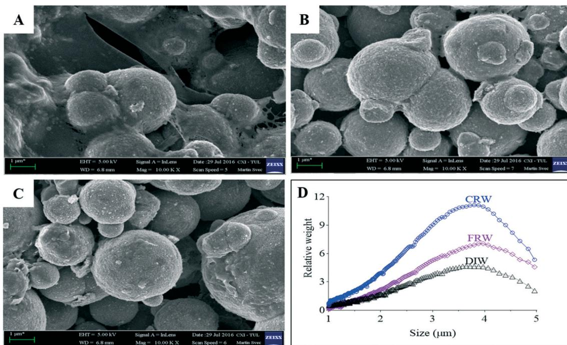
**Fig. 2** Scanning electron microscopy images of mZVI exposed for 24 h in reservoir water: (A) mZVI in centrifuged reservoir water (CRW); (B) mZVI in filtered reservoir water (FRW); (C) mZVI in deionised water (DIW) used as a control; scale bar = 1 μm; (D) size distribution of mZVI in CRW, FRW and DIW determined by differential centrifugal sedimentation.
