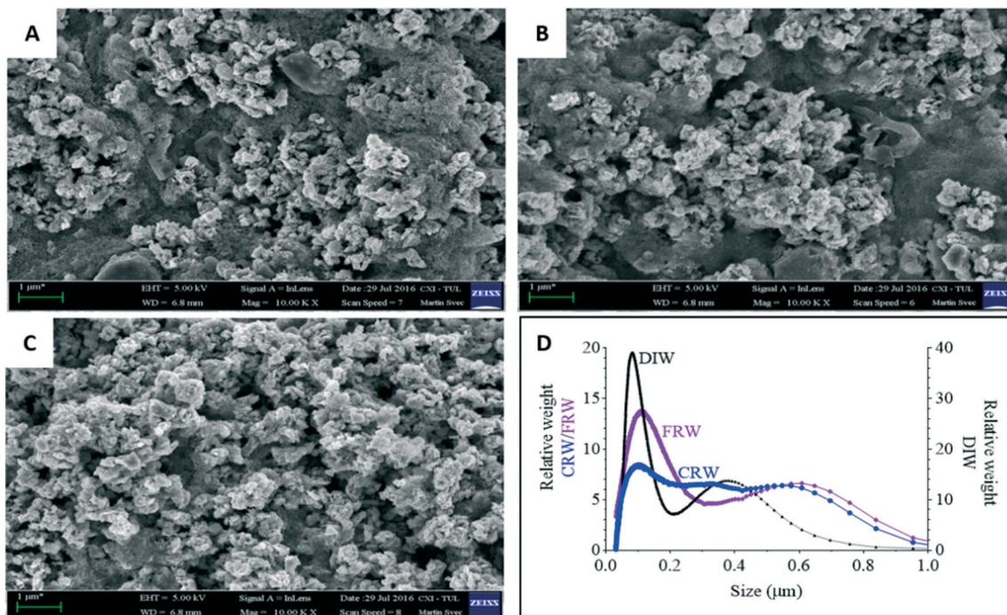
**Fig. 1** Scanning electron microscopy images of nZVI exposed for 24 h in reservoir water: (A) nZVI in centrifuged reservoir water (CRW); (B) nZVI in filtered reservoir water (FRW); (C) nZVI in deionised water (DIW) used as a control; scale bar = 1 μm; (D) size distribution of nZVI in CRW, FRW and DIW determined by differential centrifugal sedimentation.
