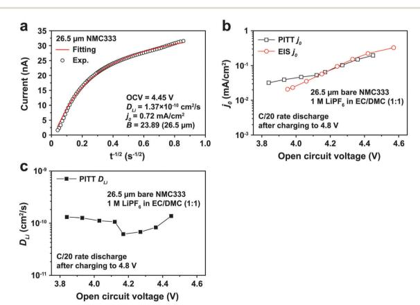
Fig. 5 (a) PITT current vs. time data, and corresponding least-squares fit to eqn (5), from which kinetic parameters are obtained, for an NMC333 particle of 26.5  $\mu$ m diameter, measured for a +15 mV voltage step from a relaxed OCV of 4.45 V. (b) The dependence of  $j_0$  on OCV from PITT (black squares) is in good agreement with those obtained from EIS (red circles). (c) Chemical diffusion coefficient  $D_{Li}$  vs. OCV, based on PITT measurements
