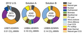
Fig. 2 Global U.S. electricity generation portfolios for 2012 (pie chart on the left), solution A (centre) and solution B (right). Slice colours represent the share of each technology according to the legend. Additionally, the associated levelised cost of electricity (LCOE, in US\$ per MWh) and the emissions rate (in CO<sub>2</sub> t per MWh) are depicted together with the pie charts.
