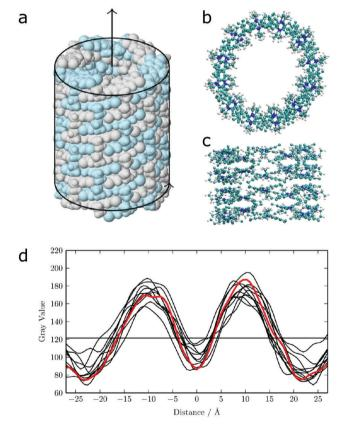
Fig. 12 (a) Idealized model for a nanotube structure of TTBC. (b) Top and (c) side view of the tube structure after MD simulations. (d) Comparison of the experimental density profile from cryo-TEM (red) with simulated 2D density profiles from 10 different angles (black lines) of the MD structure. Figure adapted from ref. 43.
