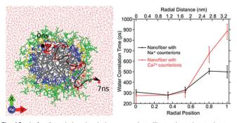
Fig. 10 Left: Atomistic simulation snapshot illustrating the trajectory (dashed line) of one water (highlighted) diffusing across the nanofiber in around 7 ns simulation time. Right: Experimentally measured water correlation time as function of the distance from the nanofiber core. Figure reproduced with permission from ref. 45. Copyright 2017 American Chemical Society
