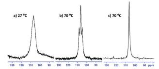
(a and b)  $^{27}$ Al NMR spectra of **3**; a triplet resolves at 70 °C,  $^{1}J_{Al-H}$  = Fig. 3 173.6 Hz. (c) <sup>27</sup>Al{<sup>1</sup>H} NMR experiment shows the triplet has collapsed to a
