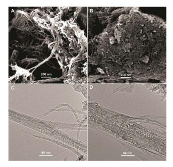
Fig. 1 SEM (A, B) and TEM (C, D) images of ABTS-PDDA/CNTs (A, C) and ABTS-PDDA/CNTs-NKB (B, D) composites.
