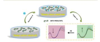
Scheme 1 Combined determination of Cu<sup>2+</sup> and β-amyloid peptide based on the ratiometric ABTS-PDDA/CNTs-NKB biosensor.
