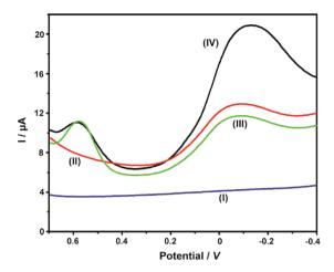
Fig. 2 DPV curves obtained on bare GC (I), PDDA/CNTs-GC (II), ABTS-PDDA/CNTs-GC (III) and ABTS-PDDA/CNTs-NKB-GC (IV) in the 100 mM PBS buffer solution containing 8.0 μM Cu<sup>2+</sup>.
