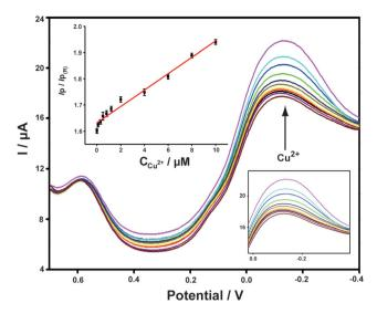
Fig. 3 DPV curves of the ABTS-PDDA/CNTs-NKB-GC toward successive additions of Cu<sup>2+</sup> at the concentrations of 0, 0.1, 0.3, 0.5, 0.8, 1.2, 2.0, 4.0, 6.0, 8.0, and 10.0  $\mu$ M. The inset is the corresponding linear plot of the  $I_P/I_{P(R)}$  ratios versus the absolute concentrations of Cu<sup>2+</sup>
