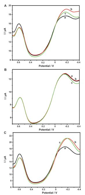
Fig. 4 DPV curves obtained on ABTS-PDDA/CNTs-NKB-GC toward 1.8 (red curve, b) and 3.8  $\mu$ g mL<sup>-1</sup> A $\beta_{1-42}$  (green curve, c) in the presence (A) and absence (B) of 6.0  $\mu$ M Cu<sup>2+</sup> PBS buffer. (C) The DPV responses of 10  $\mu$ L NaOH additions (b and c) to 6.0  $\mu$ M Cu<sup>2+</sup> PBS buffer.
