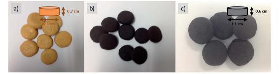
Fig. 4 Doughs obtained from glucose-urea-ZnCl<sub>2</sub>/H<sub>2</sub>O + 39% cellulose before and after baking (a) viscoelastic pellets of the dough, (b) pellets pre-baked at 100 °C for 3 hours, the green body, and (c) carbonaceous pellets made at 500 °C in nitrogen atmosphere.
