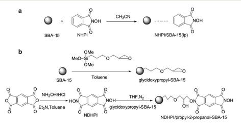
Fig. 42 The synthesis routes, (a) for NHPI/SBA-15 (ip) and (b) for NDHPI/propyl-2-propanol-SBA-15. Reprinted from ref. 171 with permission of Springer.
