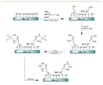
Fig. 17 Schematic diagram of SBA-15/AO/Pd(II) and SBA-15/AO/Pd(O) fabrications. Reprinted from ref. 113 with permission of Elsevier.
