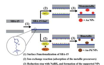
Fig. 29 Schematic illustration of the procedure carried out for the in situ synthesis of the supported mono- and bimetallic nanoparticles.
