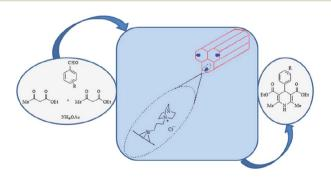
Fig. 33 Application of SBA-DABCO as basic mesoporous catalyst for the synthesis of DHP derivatives. Reprinted from ref. 155 with permission of Elsevier.
