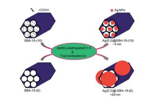
Fig. 27 Schematic illustration of the synthesis of  $Ag(y) \otimes BA-15-(x)$  nanocatalysts. Reprinted from ref. 129 with permission of Royal Society of Chemistry.
