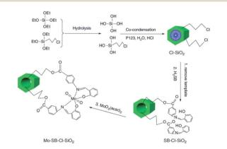
Fig. 1 Preparation of ordered Mo–SB–Cl–SiO<sub>2</sub>. Adapted from Zhang et al. (2016), ref. 92, with permission from CSIRO Publishing.
