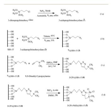
Fig. 12 (a) Synthesis of 3-azidopropyltrimethoxysilane 2. (b) Azide functionalization over SBA-15 [N $_3$ @SBA-15 3]. (c) Cycloaddition of N,N-dimethyl-2-propynylamine and N $_3$ @SBA-15 3 via the click reaction [D-2PA@SBA-15 4]. (d) Metallation of D-2PA@SBA-15 4 by PdCl $_2$  [D-2PA-Pd( $_1$ )@SBA-15 5]. Reprinted from ref. 106 with permission of Springer.
