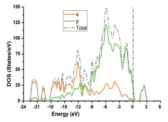
Fig. 6 Computed total density of state for NDG compound 1 and contributions from s and p orbitals.
