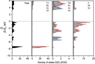
Fig. 10 Calculated total (TDOS) and partial density of states (PDOS) for (a)  $CsGaS_2-mC64$  and (b)  $CsGaS_2-mC16$ .
