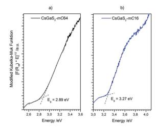
Fig. 9 Diffuse reflectance spectrum of (a) CsGaS2-mC64 and (b) CsGaS2-mC16. Optical band gaps were determined by extrapolation of the linear part of the modified Kubelka-Munk function onto the baseline, as indicated by the dashed lines.
