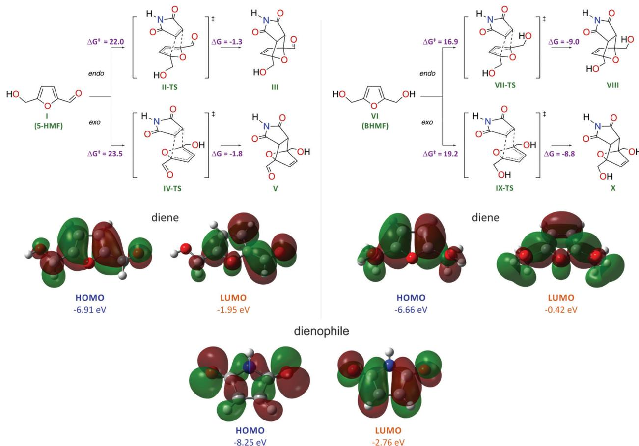
**Scheme 2** Schemes of the cycloaddition reactions for HMF and BHMF and representations of the frontier molecular orbitals for the reagents. Gibbs activation energies ( $\Delta G^\ddagger$ , kcal mol<sup>-1</sup>) and Gibbs reaction energies ( $\Delta G$ , kcal mol<sup>-1</sup>) are shown; theory level: PBE1PBE/6-311++G(d,p), GD3BJ and SCRFF (SMD, water).
