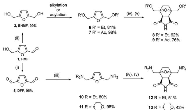
**Scheme 4** Synthesis of the norcantharimide derivatives. (i) [Pip<sup>+</sup>(O)][BF<sub>4</sub>], [BMIm][Cl]; (ii) NaBH<sub>4</sub>, water; (iii) HNET<sub>2</sub> or morpholine, STAB; (iv) maleimide; and (v) H<sub>2</sub>, 1 atm, 10% Pd/C.
