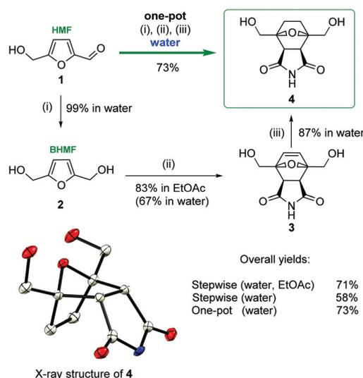
**Scheme 3** Synthesis of bis(hydroxymethyl)norcantharimide **4** in water. (i)  $\text{NaBH}_4$ , water; (ii) maleimide, water; and (iii)  $\text{H}_2$ , 1 atm, 10% Pd/C or Ni/Ra, water. Single-crystal X-ray structure of bis(hydroxymethyl)norcantharimide **4**.
