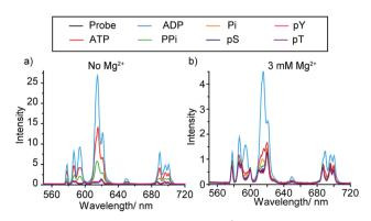
Fig. 2 Change in emission spectra of  $[Eu.1]^+$  (8  $\mu$ M) in the presence of different phosphoanions (1 mM, sodium salts) in buffered aqueous solution (10 mM HEPES, pH 7.0), containing: (a) no Mg<sup>2+</sup> ions; (b) 3 mM Mg<sup>2+</sup> ions.  $\lambda_{\rm exc}$  = 330 nm, 298 K.
