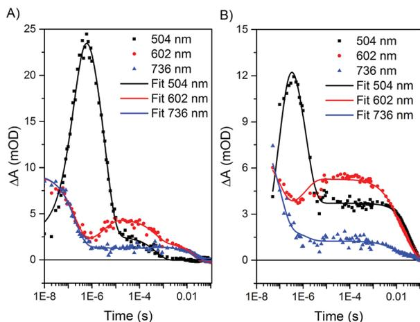
**Fig. 6** Kinetic fits of transient optical kinetic data for the (A) Ru–ApoFld–CoBF<sub>2</sub> and (B) Ru–Fd–CoBF<sub>2</sub> biohybrids with 200 mM sodium ascorbate using a global kinetic fitting routine in Origin Pro 9.1. The data sets were fit with four-exponential decay functions from 10–50 ns to 100 ms.
