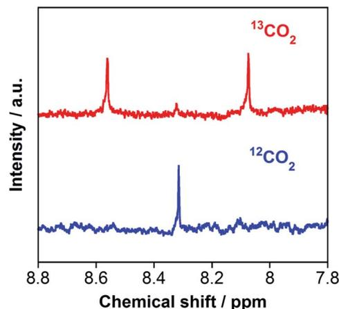
Fig. 3  $^1\text{H}$  NMR spectra of the aqueous reaction solutions (1 mL) containing  $\text{RuRu}/\text{Ag}/\text{TaON}$  (4 mg) and  $\text{EDTA}\cdot 2\text{Na}$  (10 mM), measured after 24 h irradiation at  $\lambda_{\text{ex}} > 400$  nm under  $^{13}\text{CO}_2$  (red) and  $^{12}\text{CO}_2$  (blue) atmospheres.
