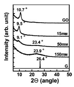
Fig. 8 XRD patterns of GO, graphite (G), and rGO obtained using various molar concentrations of NaBH $_4$ . Perinted (adapted) with permission from ref. 97. Copyright © 2009 WILEY-VCH Verlag GmbH & Co. KGaA, Weinheim.
