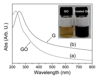
Fig. 14 UV visible absorption spectra of the GO (a) before and (b) after hydrothermal treatment at 180 °C for 6 h. Inset shows the color change of 0.5 mg mL<sup>-1</sup> GO solution before and after hydrothermal treatment.147 Reprinted (adapted) with permission from ref. 147. Copyright (2009) American Chemical Society.
