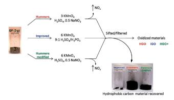
**Fig. 2** Representation of the procedures used to form GO starting with graphite flakes. Under-oxidized hydrophobic carbon material recovered during the purification of IGO, HGO, and HGO+. The increased efficiency of the IGO method is indicated by the very small amount of under-oxidized material produced.<sup>64</sup> Reprinted (adapted) with permission from ref. 64. Copyright (2010) American Chemical Society.
