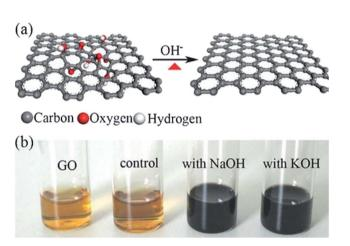
Fig. 9 (a) Illustration for the deoxygenation of exfoliated graphite oxide under alkaline conditions and (b) images of the exfoliated-graphite oxide suspension ( $\sim\!0.5~{\rm mg~mL^{-1}})$  before and after reaction. The control experiment in (b) carried out by heating the pristine exfoliated-graphite oxide suspension without NaOH and KOH at 90 °C for 5 h with the aid of sonication. Reprinted (adapted) with permission from ref. 98. Copyright © 2008 WILEY-VCH Verlag GmbH & Co. KGaA, Weinheim.
