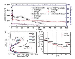
Fig. 15 (a) Cycle performance at a constant current rate of 1000 mA g<sup>-1</sup> after initial activation processes at 100 mA g<sup>-1</sup> for two cycles; (b) galvanostatic discharge-charge profiles; and (c) rate performance of Si/graphene composite electrode. 171 Reprinted (adapted) with permission from ref. 171. Copyright (2015) American Chemical Society.
