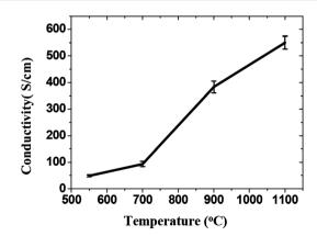
Fig. 10 Increase of the average conductivity of graphene films with temperature.<sup>111</sup> Reprinted (adapted) with permission from ref. 111. Copyright (2008) American Chemical Society.
