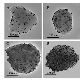
Fig. 11 TEM images of Au/g-C<sub>3</sub>N<sub>4</sub> samples with different Au loading: (A-D) 20, 60, 80 and 90 wt% (reproduced from ref. 71, licence number 3767470882063)
