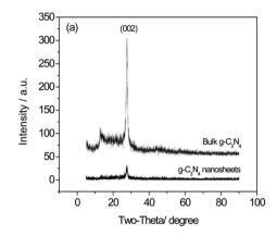
Fig. 9 XRD patterns of q-C<sub>3</sub>N<sub>4</sub> nanosheets after exfoliation (reproduced from ref. 40, licence number 3767461234354).
