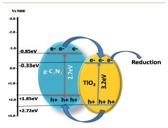
Scheme 3 Charge transfer mechanism in a heterojunction of  $g-C_3N_4$  with a wider bandgap semiconductor with both VB and CB at a higher potential.
