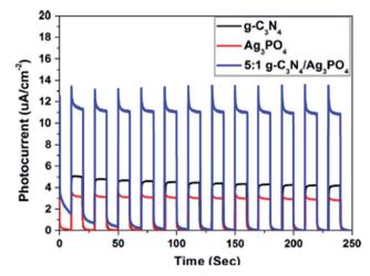
Fig. 18 Photocurrent density of 5:1 g-C<sub>3</sub>N<sub>4</sub>/Ag<sub>3</sub>PO<sub>4</sub> bulk heterojunction (reproduced from ref. 59).
