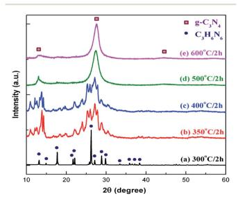
Fig. 8 XRD patterns of g-C<sub>3</sub>N<sub>4</sub> synthesized at different temperatures for 2 h (reproduced from ref. 22, licence number 3767470249553).
