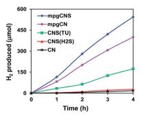
Fig. 21 Hydrogen evolution of S-doped  $g-C_3N_4$  from an aqueous solution of TEA under visible light ( $\lambda > 400$ ) (reproduced from ref. 56, licence number 3767480308846).
