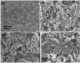
Fig. 7 SEM images of the g-C<sub>3</sub>N<sub>4</sub> synthesized at different temperatures (a) 300 °C, (b) 400 °C, (c) 500 °C and (d) 600 °C (reproduced from ref. 22, licence number 3767470249553)
