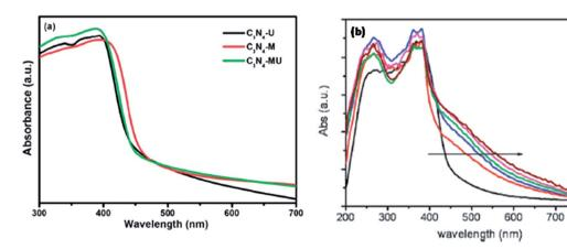
Fig. 15 (a) UV-Vis DRS of neat  $g-C_3N_4$  and (b) mesoporous  $g-C_3N_4$  prepared by using different amounts of P123 (reproduced from ref. 3 and 30).
