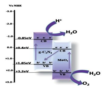
Scheme 5 Photocatalytic charge transfer by a Z-scheme mechanism.
