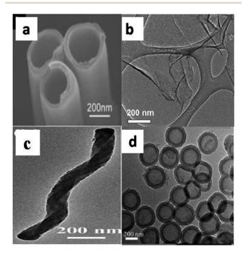
Fig. 10 TEM image of  $q-C_3N_4$  nanotubes (a), nanosheets (b), nanorods (c) and hollow nanospheres (d) (reproduced with permission from ref. 20, Copyright American chemical society, 2009, ref. 40 (licence number 3767461234354), ref. 19 (licence number 3767470642681), ref. 44).
