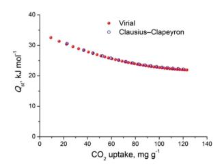
Fig. 6 CO<sub>2</sub> isosteric heat of adsorption (Q<sub>st</sub>) in Cu-PEIP as a function of surface coverage, calculated from a virial-type analysis. The corresponding Clausius-Clapeyron calculation is also shown, for comparison.
