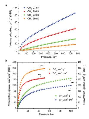
Fig. 5 (a) Low pressure CO<sub>2</sub> and CH<sub>4</sub> sorption isotherms of Cu-PEIP at the indicated temperatures, up to 1 bar. (b) The corresponding high pressure isotherms recorded at 298 K.
