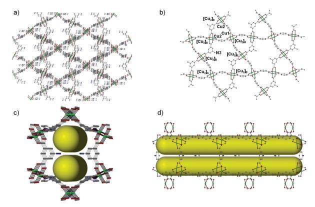
Fig. 2 Representations of (a) the 3D framework along the a axis, (b) the (3·6·3·6) semi-regular net (augmented Kagomé lattice: kgm-a), (c) the compartmentalized hexagonal channels along the a axis and (d) the compartmentalized channel projected along the a axis for complex Cu-PEIP. Colour code: Cu green, O red, N blue, C gray. H atoms are omitted for clarity.
