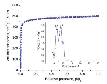
Fig. 4 Argon sorption isotherm of Cu-PEIP recorded at 87 K and pore size distribution curve calculated by NLDFT (inset).
