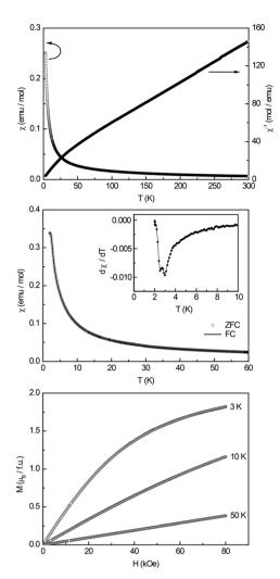
Fig. 6 Magnetic properties of Ce<sub>3</sub>Pt<sub>4</sub>Ge<sub>6</sub>: (top) Temperature dependence of the magnetic susceptibility  $\gamma$  and its reciprocal  $\gamma^{-1}$  measured with a magnetic field strength of 10 kOe; (middle) magnetic susceptibility in zero-field (ZFC) and field-cooled (FC) mode at 100 Oe; (bottom) magnetization isotherms at 3, 10, and 50 K.
