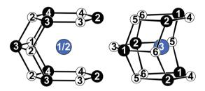
Fig. 4 Coordination environments surrounding the Ce1/2 (left) and Ce3 (right) atoms in the crystal structure of  $Ce_3Pt_4Ge_6$ . Ce atoms are depicted as blue, Pt atoms as black and Ge atoms as open white circles.
