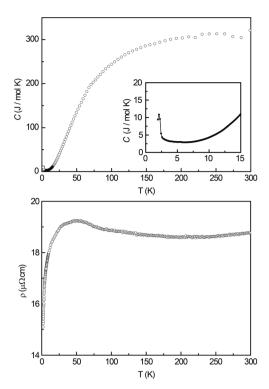
Fig. 7 Physical properties of Ce<sub>3</sub>Pt<sub>4</sub>Ge<sub>6</sub>: (top) Heat capacity measurement in the temperature range of 1.9-300 K, the inset shows the low temperature region between 1.9-15 K, indicating a  $\lambda$ -shaped anomaly; (bottom) temperature dependent electrical resistivity  $\rho$ .
