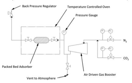
Fig. 3 Process flow diagram of high pressure testing apparatus.
