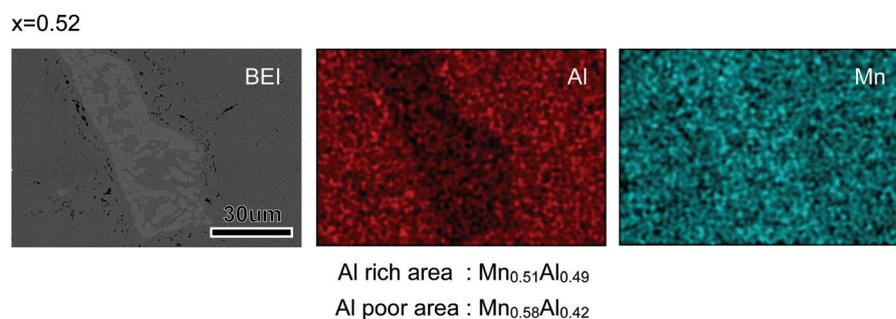
Fig. 3 Microstructural images of a  $Mn_{0.52}Al_{0.48}$  sample. Back-scattered electron image (BEI), EDS mapping images of Al (Al) and Mn (Mn). The compositions corresponding to Al rich/poor areas are also noted. The variation of the composition was found to be 1 at%.
