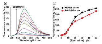
Fig. 4 (a) Fluorescence spectra of  $1-SO_3^-$  (20  $\mu M$ ) upon incubation with spermine at different concentrations (0, 2, 5, 7.5, 10, 15, 20, 30, 40, 50 μM) in artificial urine solutions at 25 °C. The spectra were obtained after incubation for 20 min. Excited at 470 nm. (b) Fluorimetric assays of spermine in HEPES buffer and in artificial urine solutions. Fluorescence intensity at 600 nm was measured as a function of [spermine].
