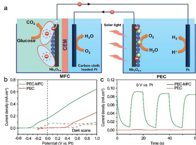
Fig. 6 (a) Schematic configuration of a PEC-MFC device; (b)  $I-V$  curves collected from a PEC device (red line) and a PEC-MFC device (olive line) with the  $\text{Nb}_2\text{O}_{5-x}$  NPs electrodes at a scan rate of  $10 \text{ mV s}^{-1}$  with/without the white light illumination; (c)  $I-T$  curves recorded for the PEC device (red line) and the PEC-MFC device (olive line) at  $0 \text{ V vs. Pt}$ , with light on/off cycles.
