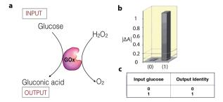
Fig. 4 (a) Schematic representation of a biocatalytic YES logic gate. (b) Bar presentation of the YES gate UV-vis absorbance outputs at  $\lambda = 500$  nm. (c) Truth table of the corresponding operation. Adapted with permission from ref. 27. Copyright (2006) American Chemical Society.
