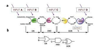
Fig. 5 Scheme illustrating the operation of concatenated logic gates based on four coupled enzyme systems. (a) Cascade of reactions catalyzed by AChE, ChOx, MP-11, and the NAD $^+$ -dependent GDH; all triggered by input signals that include acetylcholine, butyrylcholine, O<sub>2</sub>, and glucose added in different combinations. (b) Network performing OR-AND-XOR operations. Adapted with permission from ref. 30. Copyright (2006) National Academy of Sciences, U.S.A.
