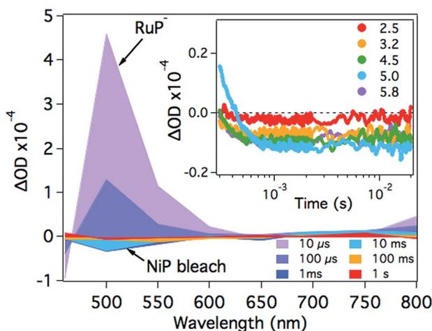
Fig. 3 Transient absorption spectra of a **RuP** (4  $\mu\text{M}$ ) and **NiP** (8  $\mu\text{M}$ ) mixture in the presence of AA (0.1 M) at pH 4.5 as a function of time delay. The inset shows the time profile of the negative signal monitored at  $\lambda = 500$  nm, assigned to the loss of ground state absorption of **NiP** in the pH range studied. The samples were excited at  $\lambda = 355$  nm.
