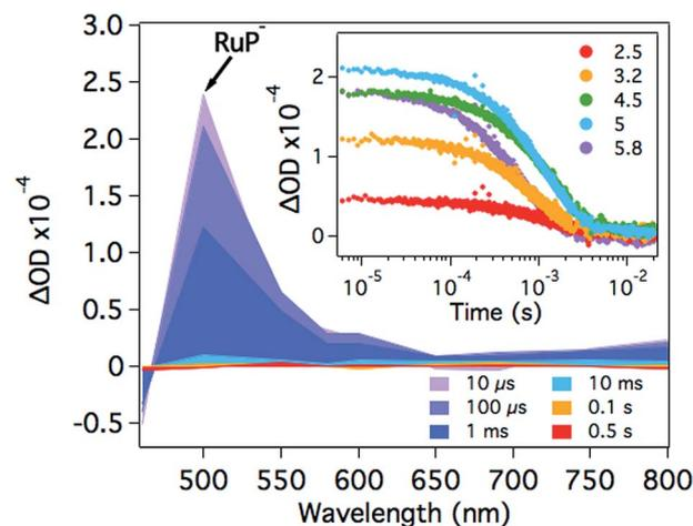
Fig. 2 Transient absorption spectra of **RuP** (4  $\mu\text{M}$ ) in the presence of AA (0.1 M) at pH 4.5 as a function of time delay. The inset shows the corresponding kinetics probed at  $\lambda = 500$  nm in the pH range between 2.5 and 5.8. The samples were excited at  $\lambda = 355$  nm.
