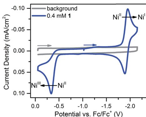
Fig. 1 Cyclic voltammogram of 0.4 mM **1** at 100 mV s<sup>-1</sup> in 0.25 M [Bu<sub>4</sub>N][PF<sub>6</sub>] acetonitrile solution. The Ni<sup>II/I</sup> couple has an  $E_{1/2}$  of  $-1.92$  V and the irreversible Ni<sup>III/II</sup> couple has an  $E_{p,a}$  of  $-0.34$  V.
