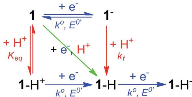
Fig. 5 Square scheme depicting possible mechanisms for addition of two electrons and one proton to compound **1**. Relevant constants are indicated.
