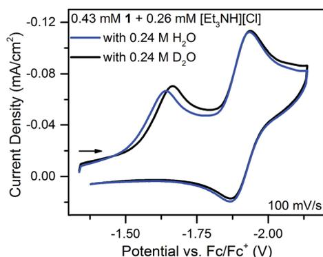
Fig. 7 Cyclic voltammograms of equimolar solutions of **1** with sub-stoichiometric [Et<sub>3</sub>NH][Cl] and either 0.24 M H<sub>2</sub>O or D<sub>2</sub>O.
