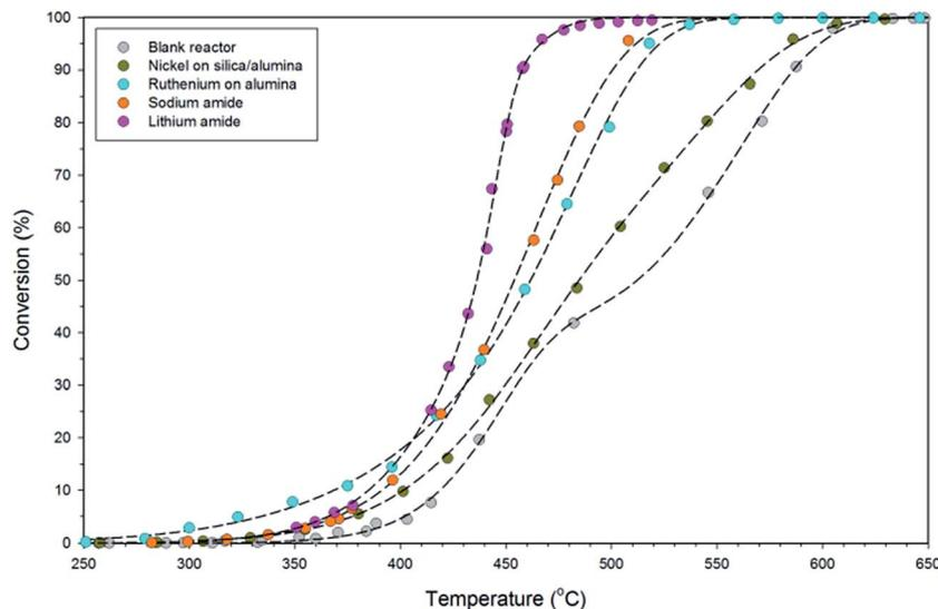
Fig. 3 Comparison of ammonia conversion as a function of reaction temperature (between 250 and 650 °C) for the blank 46.9 cm<sup>3</sup> stainless steel reactor and when containing 0.5 g of LiNH<sub>2</sub>, NaNH<sub>2</sub>, silica/alumina-supported nickel, and alumina-supported ruthenium, at an ammonia flow rate of 60 sccm, with dashed lines showing sigmoidal fits to the data.
