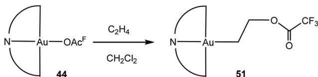
**Scheme 24** Ethylene insertion into the gold–trifluoroacetate bond.<sup>114</sup>
