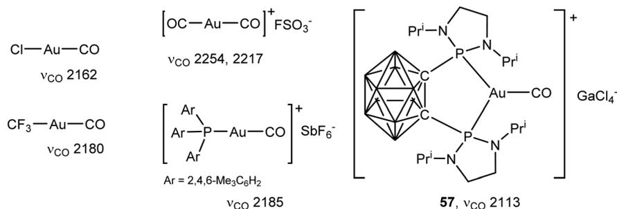
Scheme 27 Representative types of Au(I) CO complexes, with  $\nu_{\text{CO}}$  stretching frequencies (cm<sup>-1</sup>).<sup>128,129,133,138</sup>
