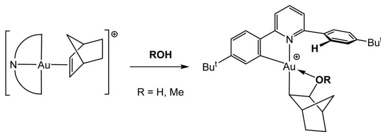
**Scheme 23** Reaction of the gold(III) norbornene complex **47** with protic reagents.<sup>114</sup>
