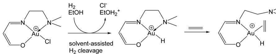
**Scheme 7** Computational models for proposed intermediates in alkene hydrogenation catalysed by Au(III) Schiff base complexes.<sup>50</sup>
