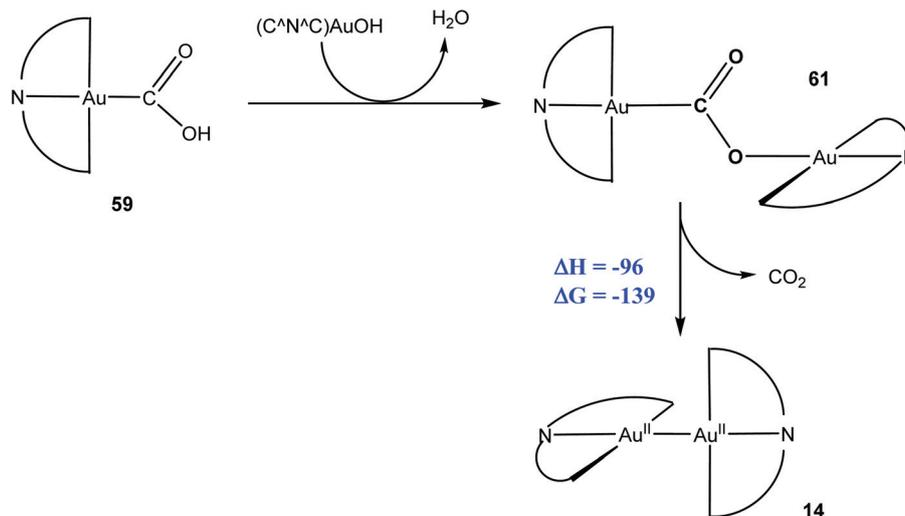
**Scheme 31** Thermally induced reductive CO<sub>2</sub> elimination from a di-gold complex. Enthalpy and Gibbs free energy values (kJ mol<sup>-1</sup>) as calculated by DFT (*T* = 298.15 K).
