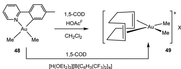
**Scheme 22** Synthesis of Au(III) COD complexes.<sup>120</sup>
