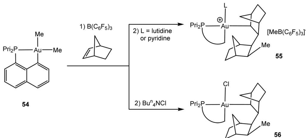
Scheme 26 Norbornene insertion into an Au–Me bond.<sup>122</sup>
