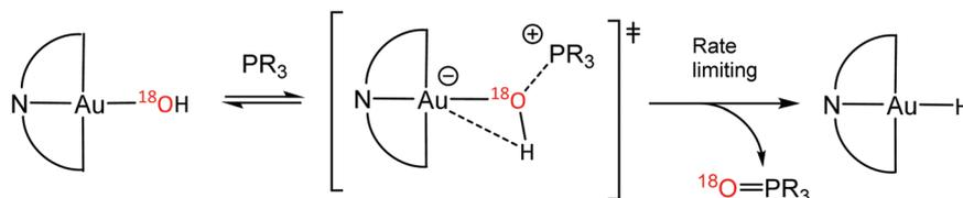
**Scheme 15** Proposed mechanism for O-abstraction from Au<sup>III</sup>-OH by phosphines.
