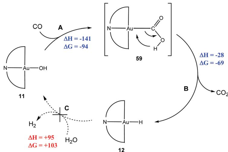
**Scheme 29** WGS-type reactions of  $(C^N^C)AuOH$ . Enthalpy and Gibbs free energy values (in  $\text{kJ mol}^{-1}$ ) for reaction steps as calculated by DFT ( $T = 298.15 \text{ K}$ ).<sup>144</sup>
