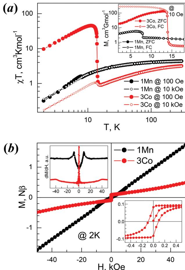
**Fig. 6** Magnetism of **1Mn** and **3Co**. (a) Plots of  $\chi T$  vs.  $T$  under 100 Oe and 10 kOe fields, (inset) the ZFC/FC plots of the **1Mn** and **3Co** under 10 Oe field. (b) Isothermal magnetization plots of **1Mn** and **3Co** at 2 K, (top-left inset) the  $dM/dH$  plots, (bottom-right inset) hysteresis loop for **3Co**.
