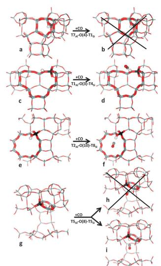
Brønsted-acid sites without and with an adsorbed CO (left and right parts, respectively) shown for Al in T7 (a, b), T1 (c, d), T2 (e, f), and T5 (g-i). Framework Si, Al, and O atoms are depicted in grey, black, and red colour, respectively, while the H atom of the Brønsted-acid OH group, and C and O atoms of CO are depicted as white, grey, and red balls, respectively
