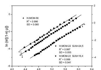
Fig. 5 Plot of the left-hand side of eqn (5) against the reciprocal of the temperature for CO adsorbed on H-MCM-22 (Si: Al = 24.5:1 and 16.4:1) and H-MCM-56; data obtained from the O-H stretching bands, R. linear regression coefficient; SD, standard deviation.
