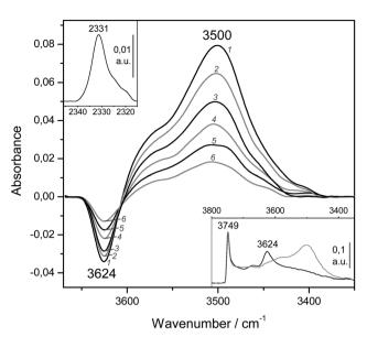
Fig. 12 Representative variable-temperature IR spectra (O–H stretching region) of  $\rm N_2$  adsorbed on H-MCM-56. The spectra are shown in the difference mode (zeolite blank subtracted). From 1 to 6, temperature goes from 145 to 174 K; and equilibrium pressure from 9.55 to 10.95 mbar. The bottom inset shows the blank zeolite spectrum (black) and the effect of dosing with  $\rm N_2$  at 77 K (grey). The top inset shows the N–N stretching region of spectrum 1.
