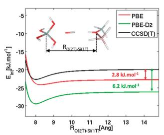
**Fig. 2** Interaction energy of CO with the Brønsted-acid site (represented by the 2T cluster model) and the model of the zeolite framework (represented by the 1T cluster model) calculated at CCSD(T), PBE, and PBE-D2 levels, as a function of the  $R_{\rm O(2T)-Si(LT)}$  distance. Framework Si, Al, O, and H atoms are depicted in grey, pink, red, and white colours, respectively, CO atoms are depicted in red and grey (O and C atom, respectively).
